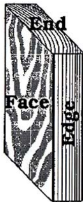
Figure 2. For purposes of clarity, herein, the different surfaces of lumber are referred to as the ends, edges and faces, without regards to grain pattern.
