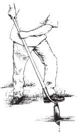
Insert a sand shovel vertically into soil.
